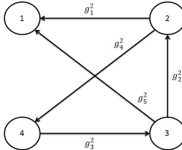
Figure 1: Information-exchange topologies between four agents (underlying graph  $\mathcal{G}$ )
