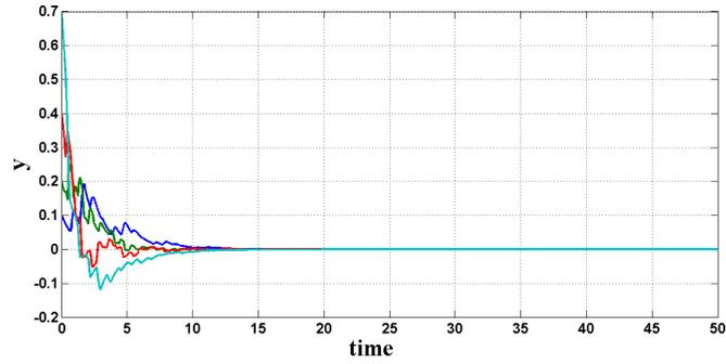
Figure 3: Velocity trajectories of the four agents
