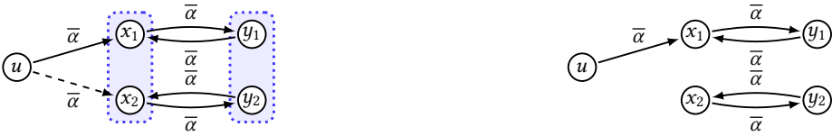
Fig. 10. A graph G where \{x_1, x_2\} and \{y_1, y_2\} are inter-reachable (left). After deleting the edge u \xrightarrow{\bar{\alpha}} x_2 , every pair of nodes are not inter-reachable (right).
