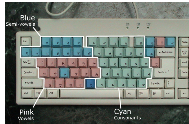
figure 4: Keylekh 1 keyboard made by using plastic parts from a commercially available QWERTY keyboard. The consonant and vowel blocks have been swapped. The colors of the blocks have been labeled for black and white reproduction.
