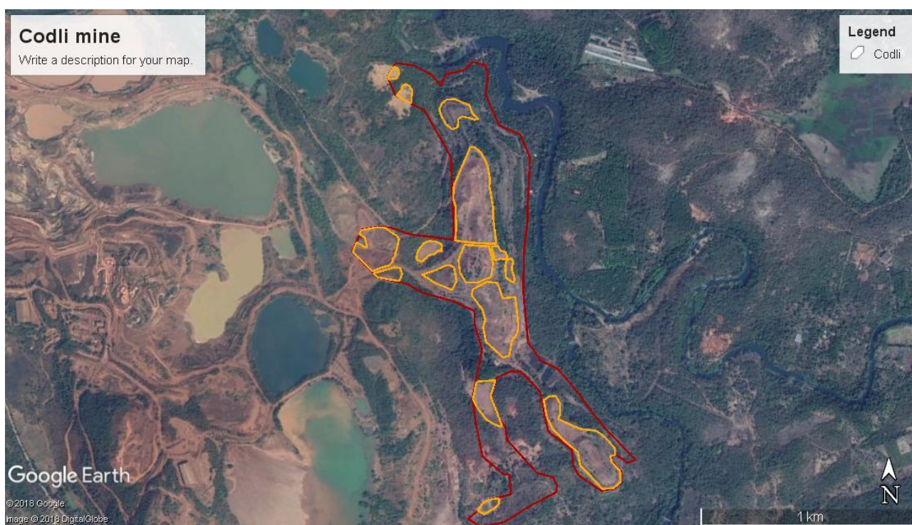
Figure 6-2 Mapping of feasible areas for solar PV in abandoned mine lands
