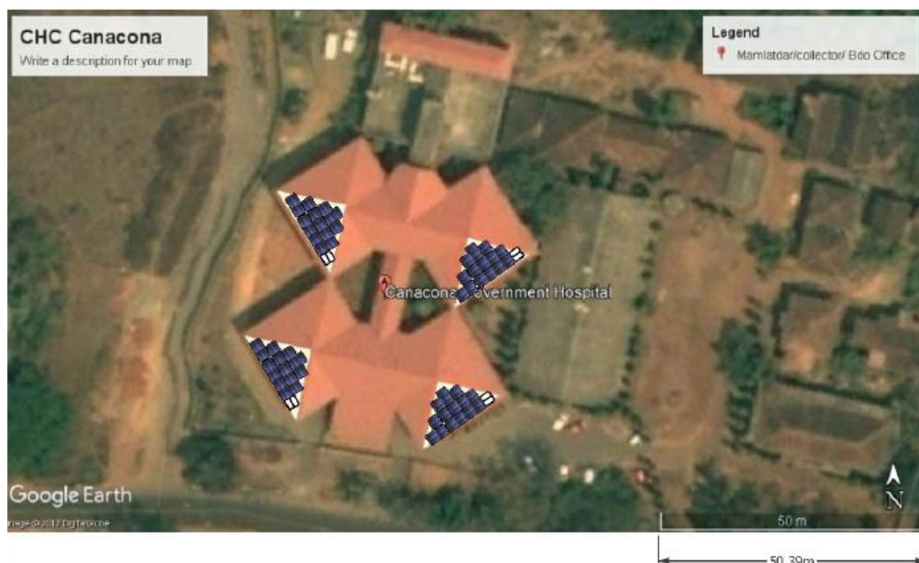
Figure 3-7 Placement of panels using Sketchup
