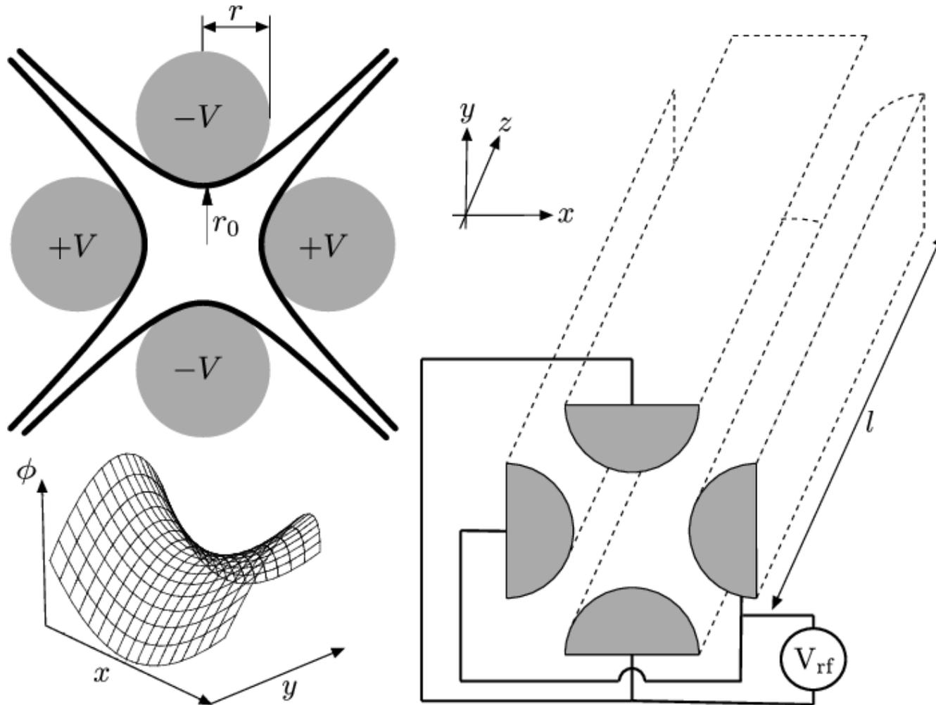
A schematic of an ideal hyperbolic electrostatic quadrupole (thick line) and the circular electrodes used to closely approximate the hyperbolic shape are shown on the top left. The saddle-shaped harmonic potential it creates is illustrated at the bottom left. The geometry formed from half-cylindrical rods and pair-wise applied a.c. potential ( $V_{rf}$ ).
