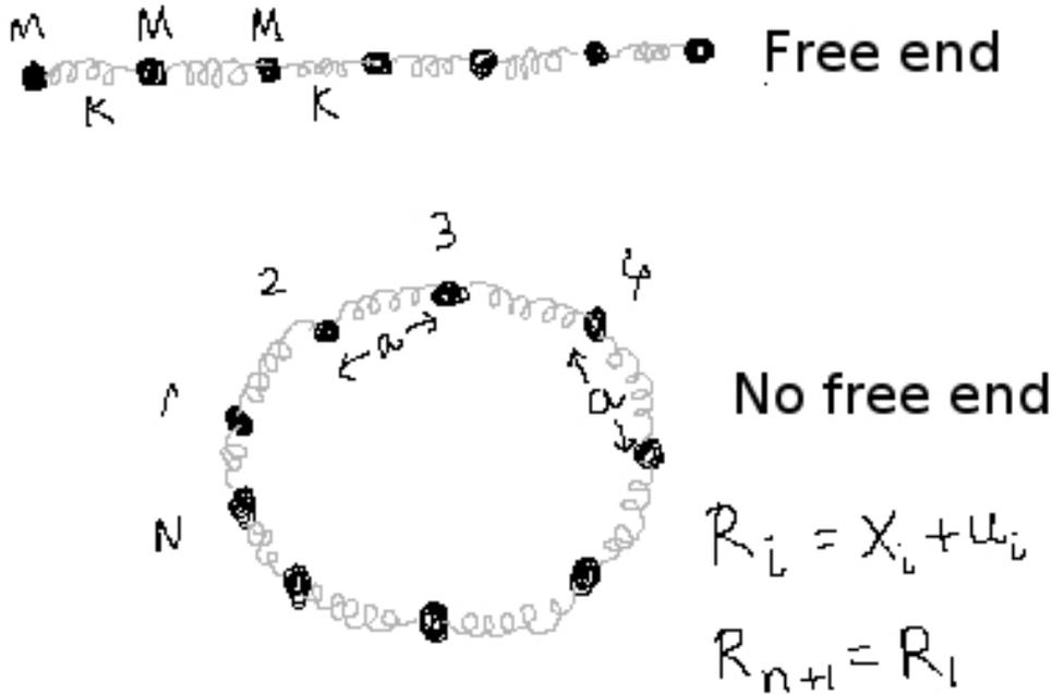
Figure 6.1: The periodic boundary condition, in 1d means using a ring rather than a line. The compression of the spring between  $i^{\text{th}}$  and  $i+1^{\text{th}}$  site is given by  $u_i - u_{i+1}$ . Note that the correct sign of the displacements is needed. Here we will consider displacements to be positive if it is to the right - following the usual convention that the x-axis is positive in the right direction. The displacements are longitudinal.
