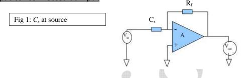
Consider the circuit of Fig 1. Notice the difference from standard inverting feedback amplifier: the *source* resistor has been replaced by a capacitor  $C_{s}$ .
