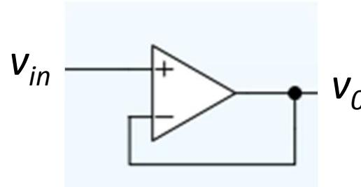
When it's cold,  $v_{in}$  falls  $\rightarrow v_o$  falls  $\rightarrow v_-$  decreases  $\rightarrow (v_+ - v_-)$  increases
