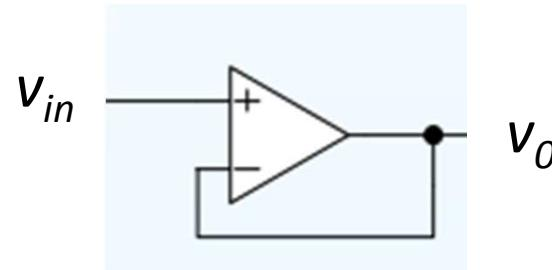
$$v_o = A(v_+ - v_-)$$
