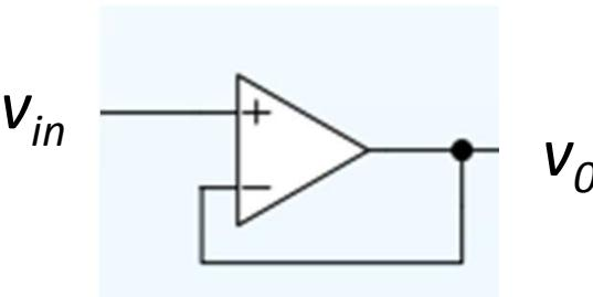
$$v_o = A(v_+ - v_-)$$
