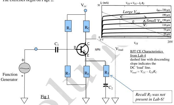
The Design Process is split in two independent parts: First we do DC design to bias the BJT in Active mode. Then the AC design is done to make the amplifier amplify AC signals.
