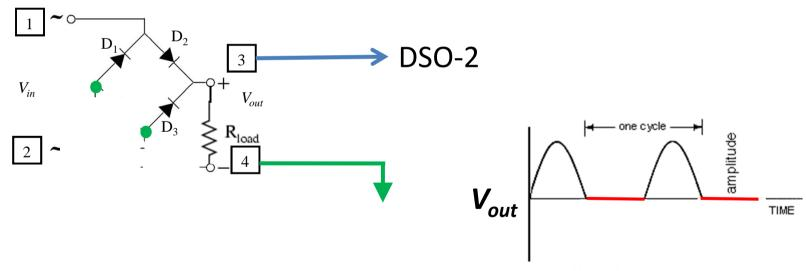
Note: D<sub>1</sub> and D<sub>3</sub> function as positive clamps (like Slide 4)
