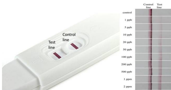
Fig. 1. Lateral Flow test Strip showing various intensities corresponding to various concentrations of Biomarker [1]
