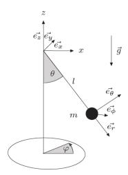
If length of the rod is l, then r=l, and  $\dot{r}=0$ , we are left with two generalized coordinates  $(\theta,\phi)$ , with
