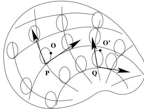
Figure 1: This shows a curved surface with a curvilinear coordinate system. Local reference axes at grid points P and at Q have different scalings. The circles shown at each grid point do not belong to the curved surface itself, but represent an auxiliary internal space. For the internal space the origin can be independently chosen at different points, e.g., O at P and O' at Q.
